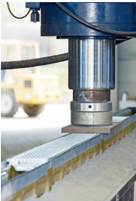
Tightness testing after long-term simulation
