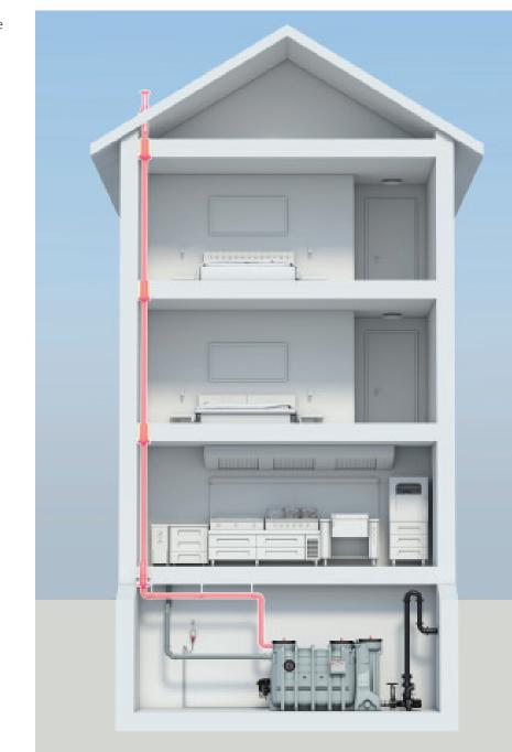
For grease separators with automated cleaning/ disposal appropriate control units for both the grease separator and the lift plant have to be specified. Moreover, some manufacturers require the installation of the control unit at the wall of the installation room.
